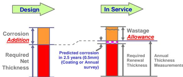
Figure 1 : Net thickness principle
