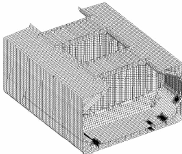
Figure 5 shows an example of the fine mesh model with very fine mesh areas imbedded within the model.
