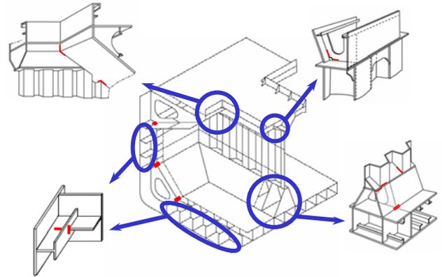
Figure 8 : Example of bulk carrier details to be checked in fatigue
