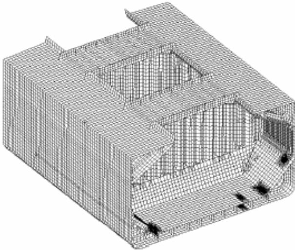
Figure 5 : Local Fine Mesh FE Model
