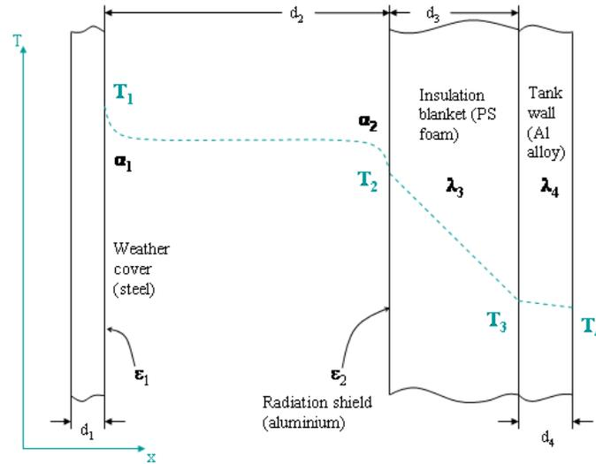
Fig. 6.1 Model of the spherical tank system,
