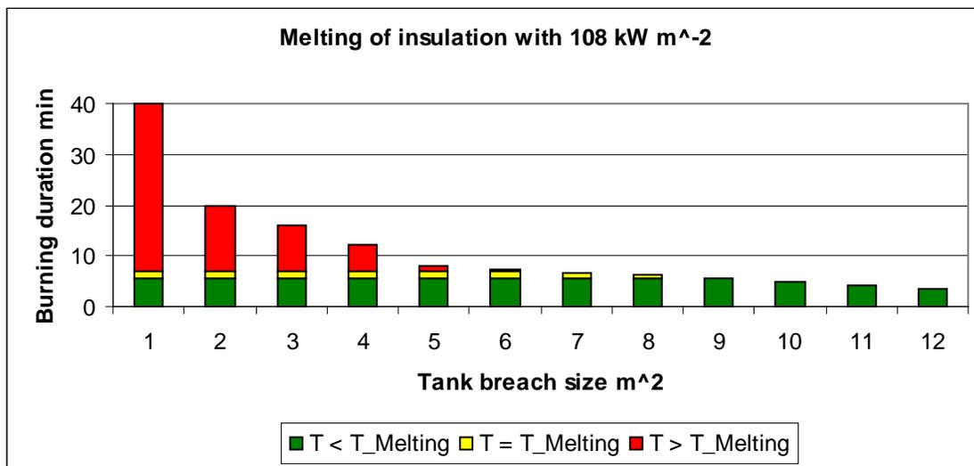
Fig. 6.9 Melting of insulation caused by a heat flux of  $108 \text{ kW m}^{-2}$ ,
