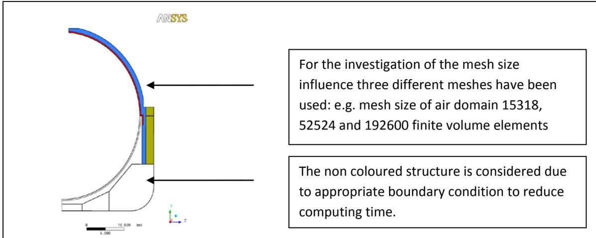
Fig. 6.4 Model of the solution domain, [10] modified
