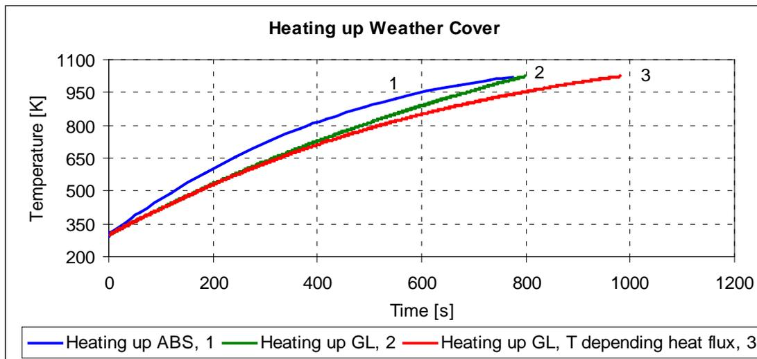
Fig. 6.6 Comparison heating up the weather cover ABS / GL
