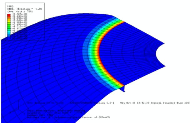
Fig. 6.5 Location of the thermal collapse (buckling),
