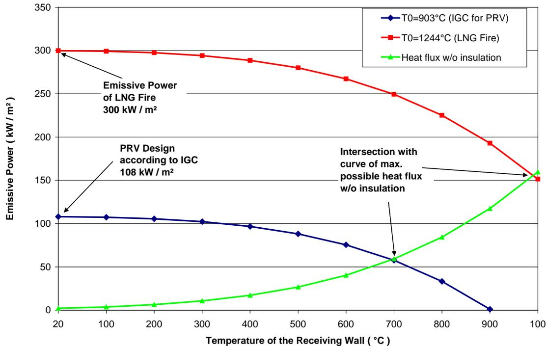
Fig. 6.2 Maximum heat flux (or emissive power) into the tank
