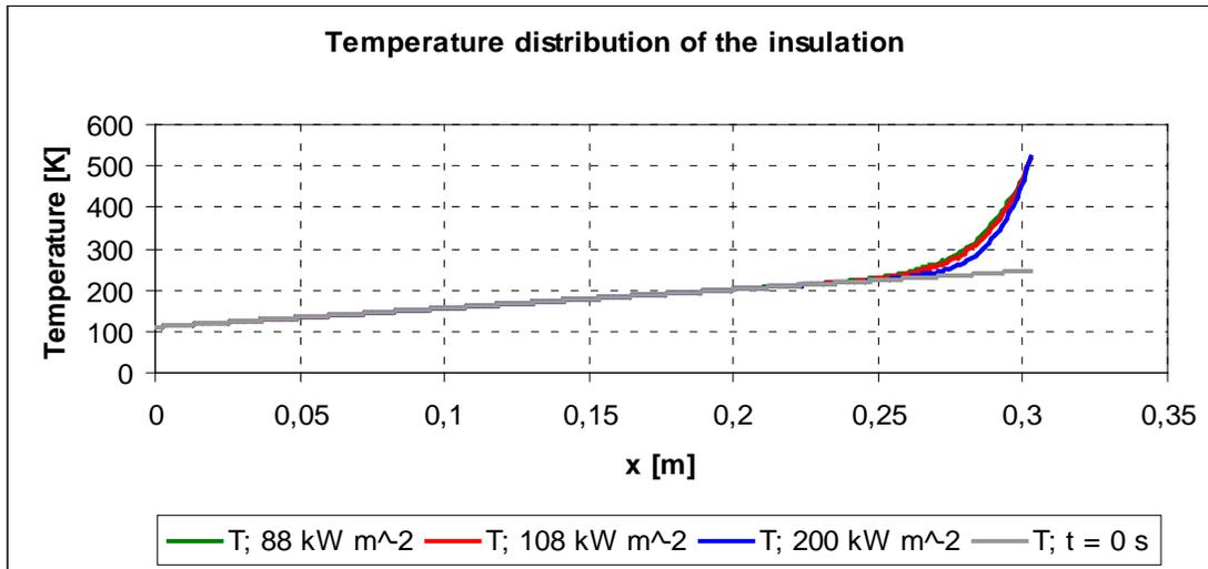
Fig. 6.8 Temperature distribution inside cross section of the insulation, [10] modified
