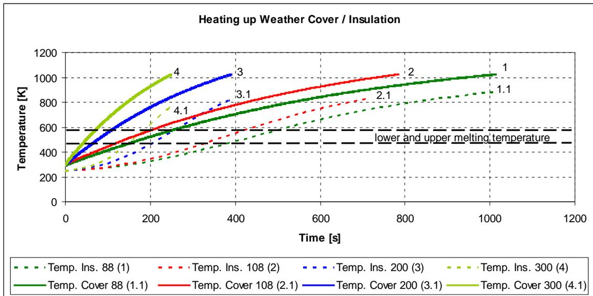
Fig.6.7 Heating up of the weather cover and insulation,
