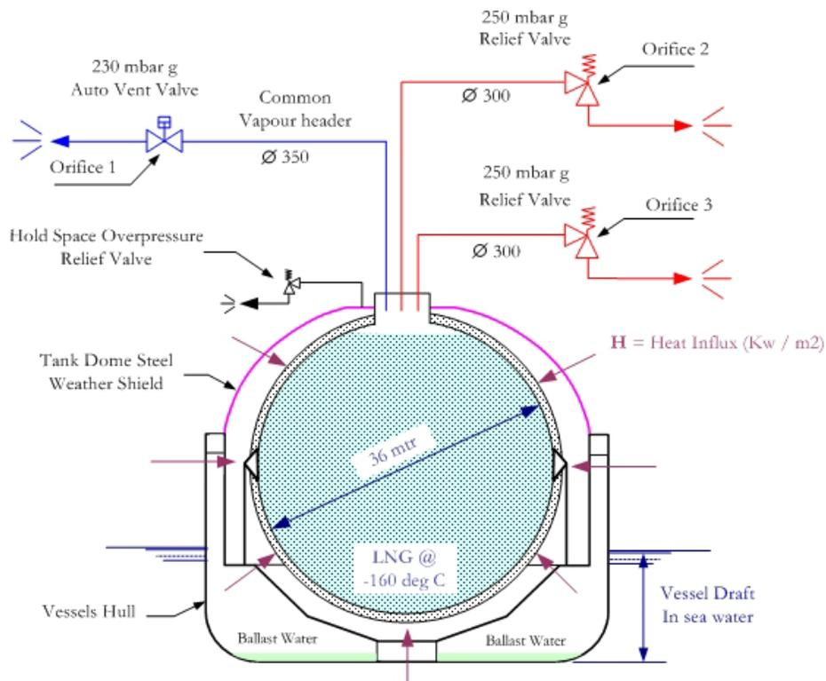
Fig 5.1 Cross section of relief system for a Moss tank
