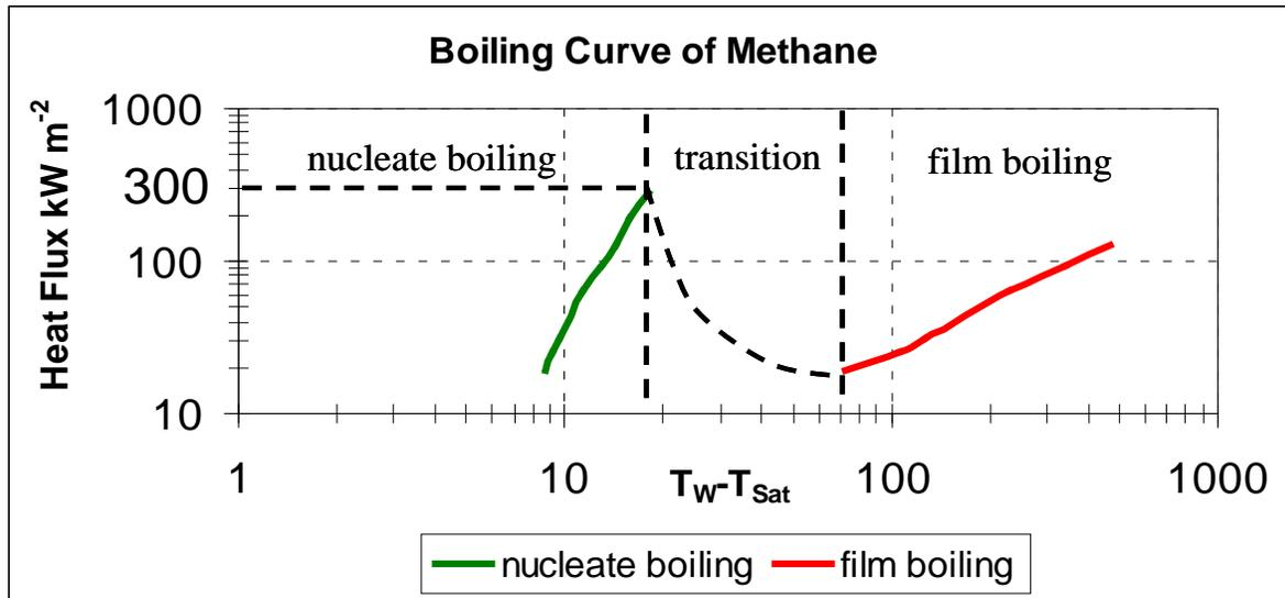
Fig. 6.3 Boiling curve of methane,
